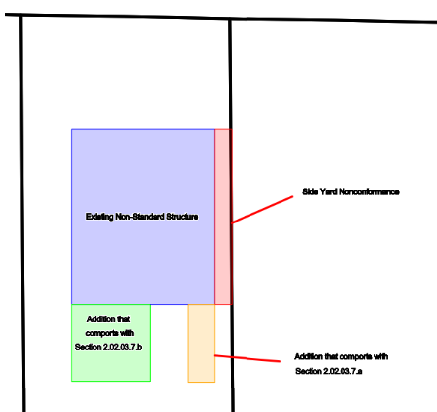
Figure 2.02.03 Example of Addition to a Non-Standard Structure
