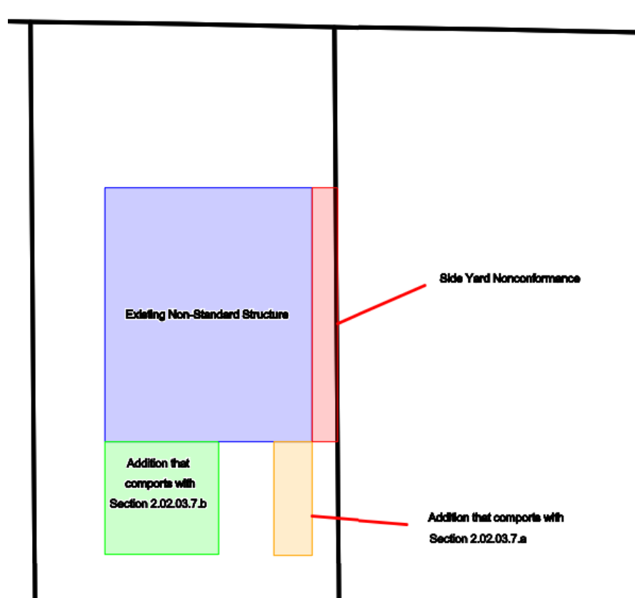
Figure 2.02.03 Example of Addition to a Non-Standard Structure
